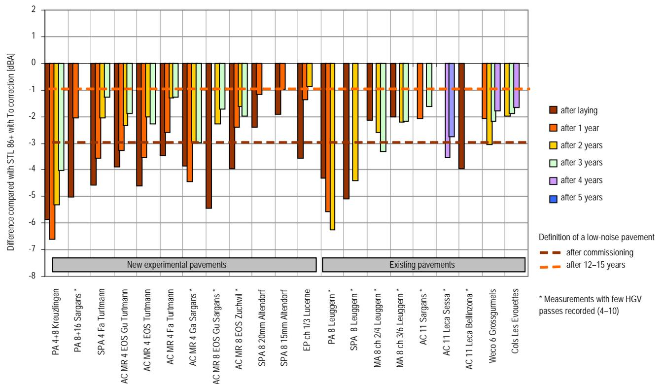
Acoustic performance decreased in a more or less marked fashion for all the new experimental pavements and most of the existing pavements. In the first 3 years, the decrease in performance was between 1 and 3 dBA, though this became less pronounced in the third year. Of the newly laid, semi-dense pavements, the AC MR 4 pavement in Sargans exhibited the best acoustic performance after 3 years.
